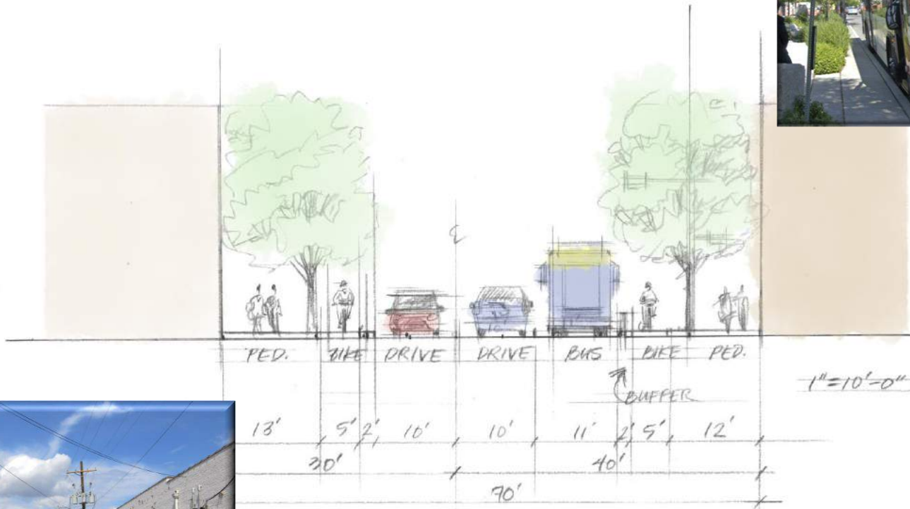
14th Street with Bike Lane PROPOSED CROSS SECTION
